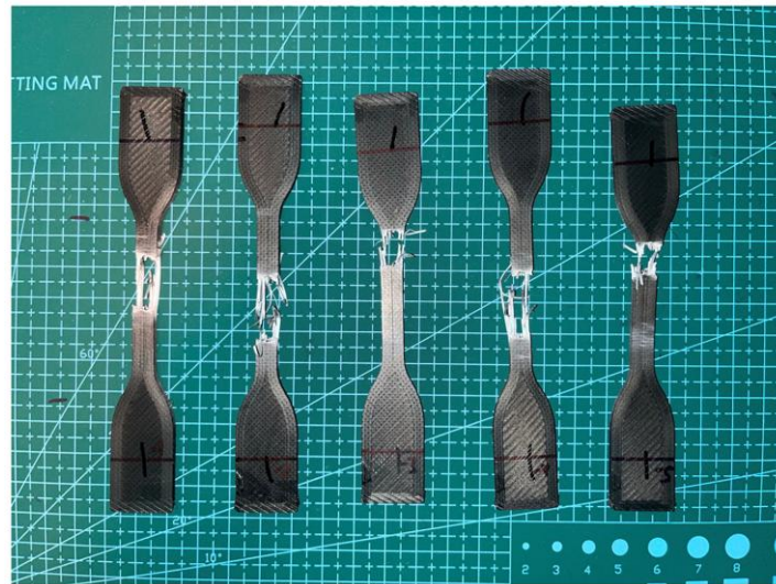
Fig 4 . Sample Run 1 after the tensile test (layer thickness = 0.2 mm, printing speed = 30 mm/s, infill density = 20%)
