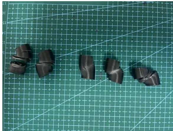
Fig 6 . Sample 2 after the compressive test (layer thickness = 0.2 mm, printing speed = 30 mm/s, and infill density = 20%)
